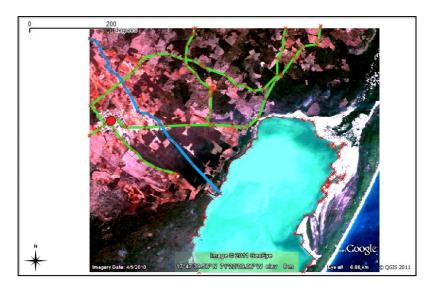
Pictured below are the **digitised features** saved as a number of shapefile layers, the Google Earth base image has been removed. This data can now be used in your project to construct a map fit for purpose.
